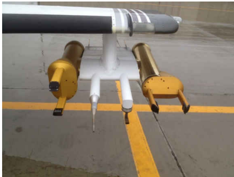
Figure 3: The configuration of the inboard vertically mounted High Volume Precipitation Spectrometer Version 3 (HVPS-3) (left) and outboard horizontally mounted HVPS-3 (right). The orientation of the outboard HVPS-3 was modified depending on the day.
