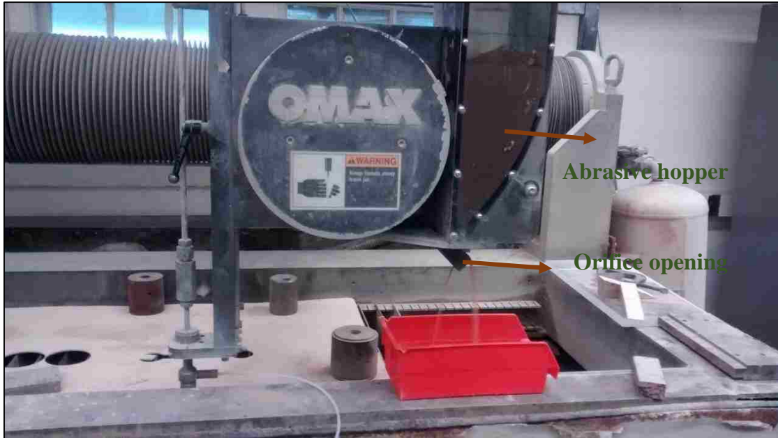
Figure 4.9. OMAX waterjet systems gravity controlled abrasive feeder
