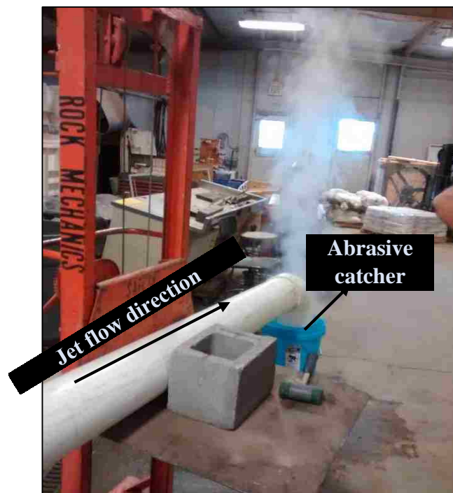
Figure 4.11. Abrasive capture after jet exit
