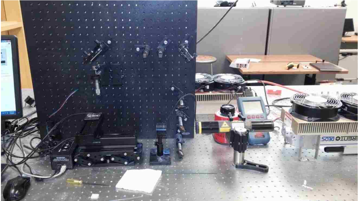
Figure 1.1. Glass AM Prototype System Without the Prototype Wire Feeder Mounted.
