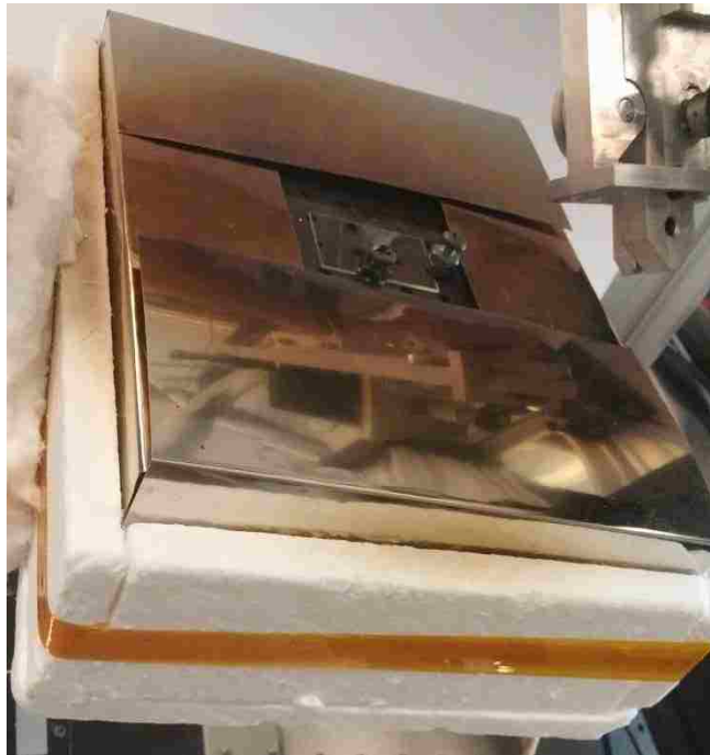
Figure 2.7. The Substrate Heater with a Soda-Lime Glass Slide Bolted Into Place on the Build Platform.
