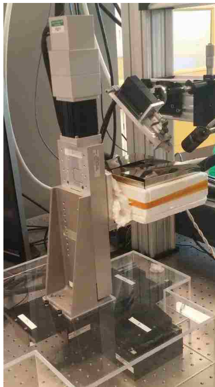
Figure 2.6. Aerotech Stages used in the Glass AM Process with the Substrate heater attached.
