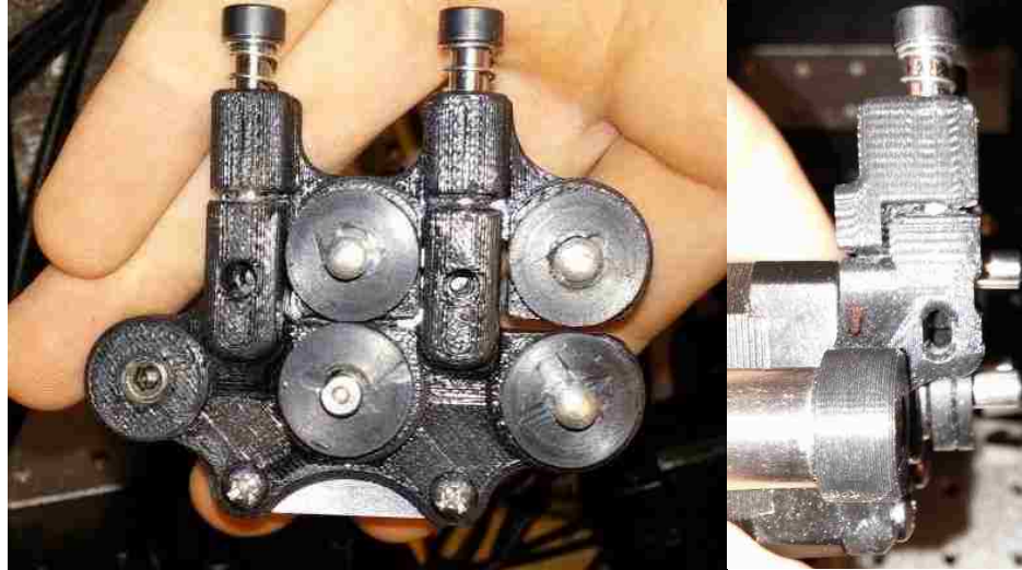
Figure 1.2. A Front and Side View of the Wire Feeding Mechanism. The bottom left wheel is powered by a bipolar stepper motor and the top piece is held in place by two shoulder bolts which are screwed into tapped holes in the thermoplastic bottom piece. The picture on the right shows the wire feeder rotated 90 degrees to show the mounting mechanism, the hole through which glass was fed, and the groove in the wheels.
