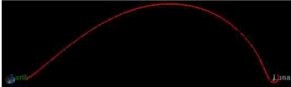
Figure 4.6. The Perilune 1 trajectory simulated in GMAT, beginning at disposal from the ICPS, and viewed along the negative Z direction of the X-Y projection of the Earth-Moon rotating frame.
