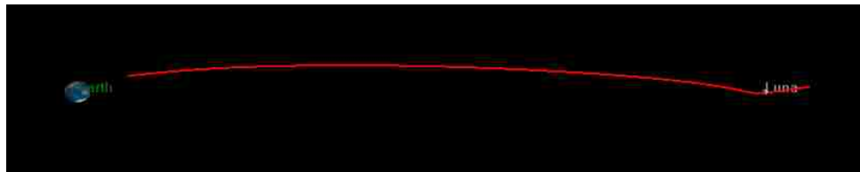
Figure 4.3. The ballistic trajectory simulated in GMAT, beginning at disposal from the ICPS, and viewed along the positive Y direction of the X-Z projection of the Earth-Moon rotating frame.
