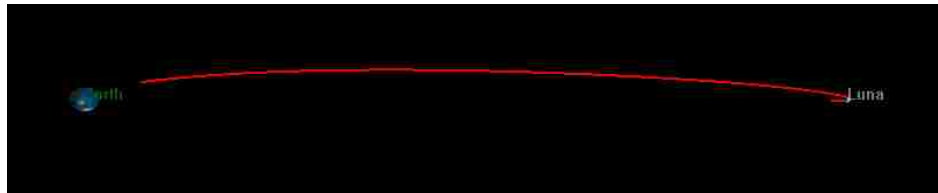
Figure 4.23. The Van Allen 2 trajectory simulated in GMAT, beginning at disposal from the ICPS, and viewed along the positive Y direction of the X-Z projection of the Earth-Moon rotating frame.
