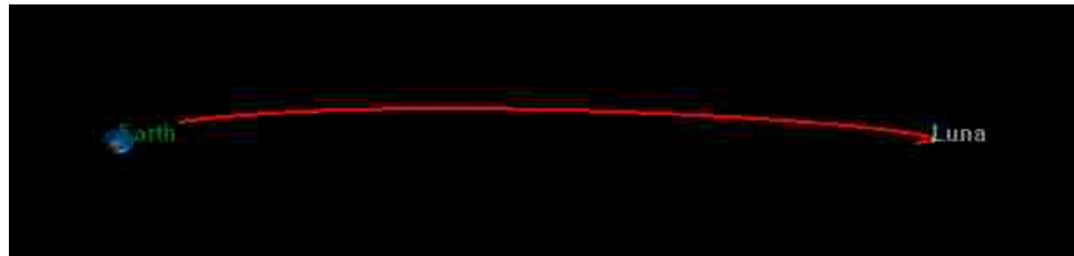
Figure 4.15. The Disposal 2 trajectory simulated in GMAT, beginning at disposal from the ICPS, and viewed along the positive Y direction of the X-Z projection of the Earth-Moon rotating frame.
