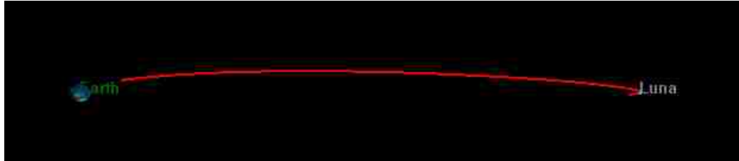
Figure 4.14. The Disposal 2 trajectory simulated in GMAT, beginning at disposal from the ICPS, and viewed along the negative Z direction of the X-Y projection of the Earth-Moon rotating frame.
