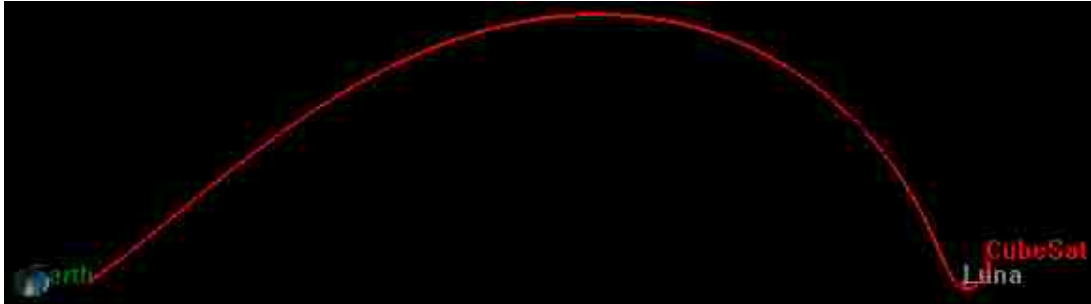
Figure 4.19. The Van Allen 1 trajectory simulated in GMAT, beginning at disposal from the ICPS, and viewed along the negative Z direction of the X-Y projection of the Earth-Moon rotating frame.
