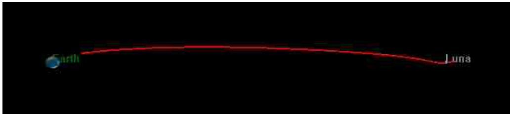
Figure 4.7. The Perilune 1 trajectory simulated in GMAT, beginning at disposal from the ICPS, and viewed along the positive Y direction of the X-Z projection of the Earth-Moon rotating frame.
