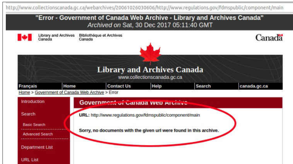
Fig. 65: The Canadian archive responds with soft 404 to the request of a memento that is not available in the archive (i.e., returning 200 OK with an HTTP entity indicating that the resource is not in the archive).
