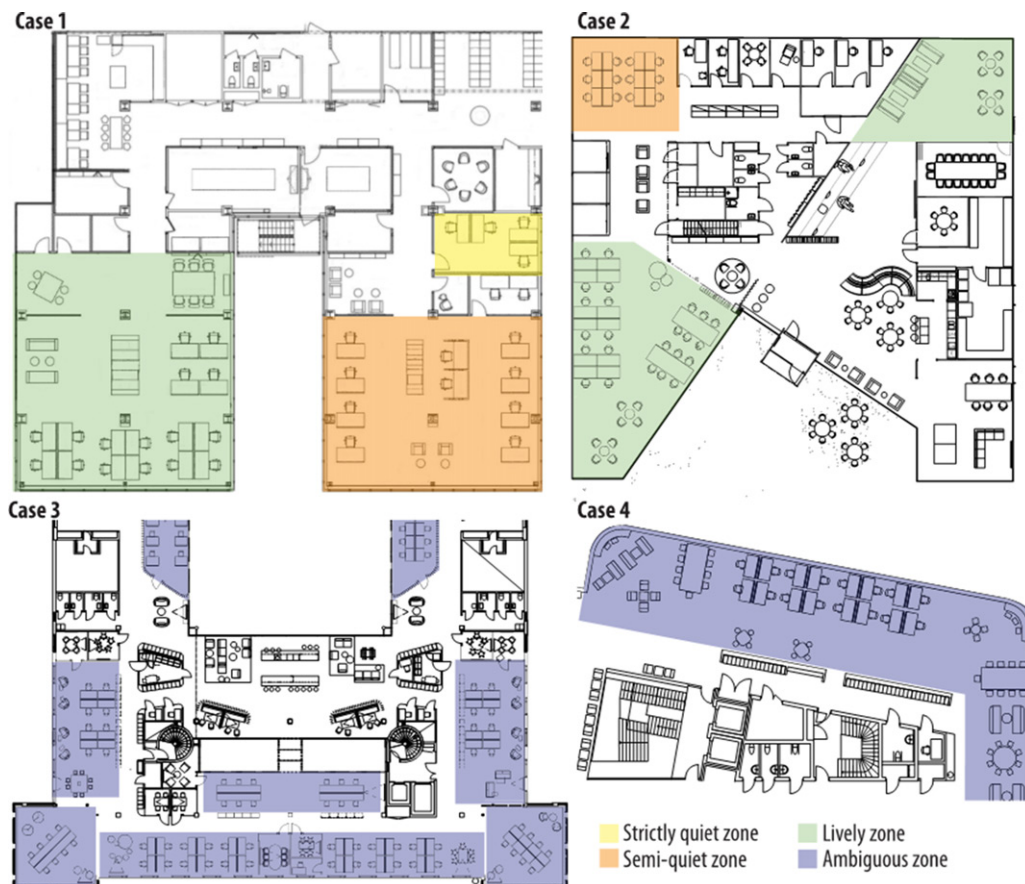
Figure 1. Architectural drawings marked with allocated zones for different speech levels.
