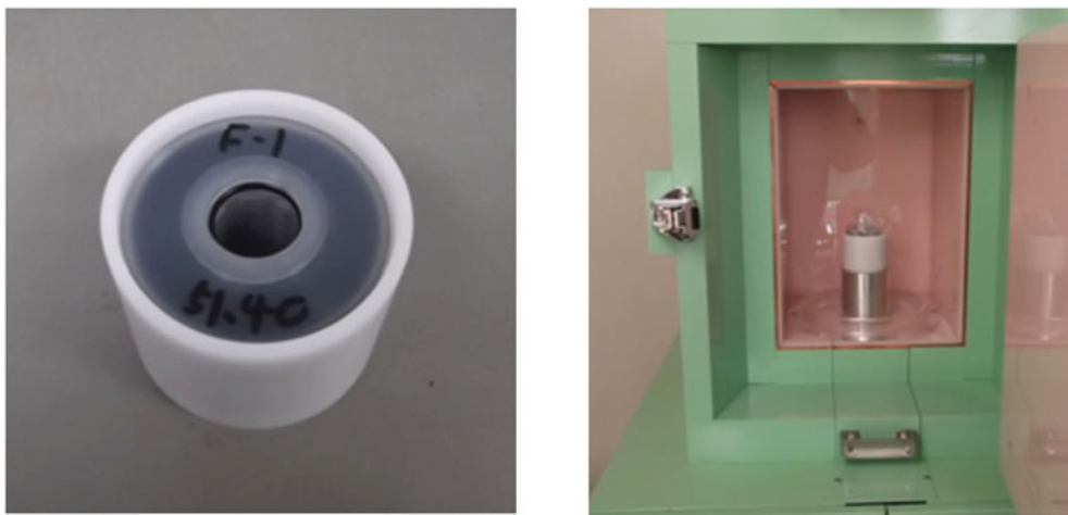
Photo 1. PBC and plastic case for direct measurement of ^{137}\text{Cs} concentrations by Ge semiconductor detector (left) and measurement situation of PBC with plastic case by Ge semiconductor detector (right).
