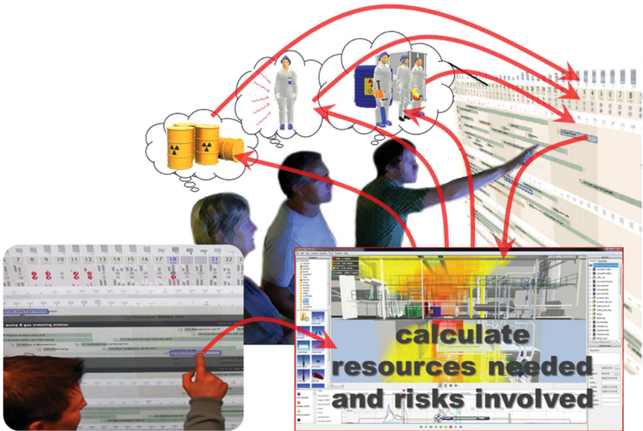
Figure 5. Scheduling work tasks and allocating resources by combining the results of 3D work simulation, to determine the details of jobs, and an interactive visual overview of the overall schedule, used to coordinate jobs taking into account safety and resource constraints.
