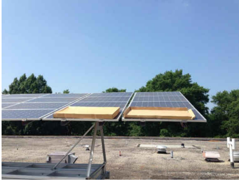
Figure 3.17: Shading arrangement for two shaded PV modules.
