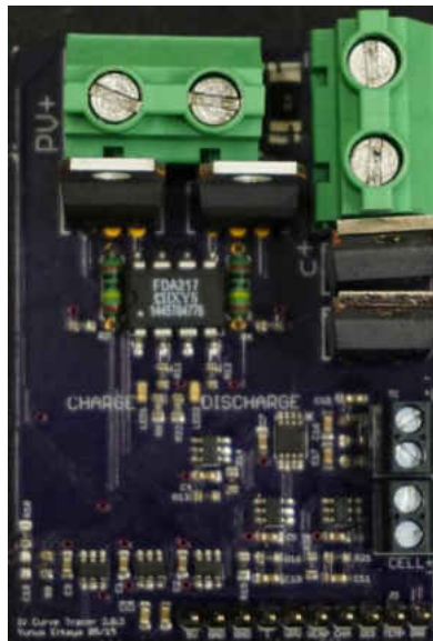
Figure 3.28: I-V curve tracer circuit board after assembly.
