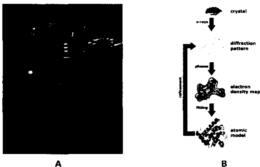
Figure 5. Two experimental methods to determine protein 3-D structure. (A) A 900MHz NMR instrument with a 21.2 T magnet at HWB-NMR, Birmingham, UK, Courtesy of Martin Saunders. (B) Workflow for solving the structure of a molecule by X-ray crystallography. Courtesy of Thomas Splettstoesser.
