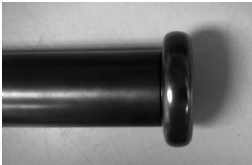
Figure 2-10. Photograph of endcap on solid cathode [5].
