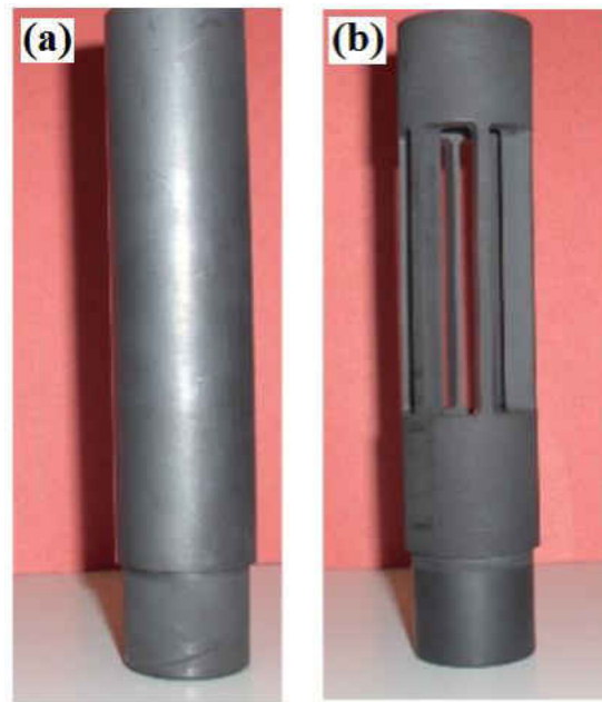
Figure 2-13. Two different types of cathode produced at UNM. (a) Solid cathode. (b) Transparent cathode [2].
