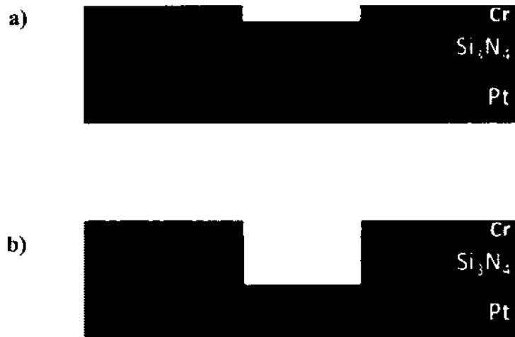
Figure 22. Schematic showing pattern transfer using the Cr hard mask a) before and b) after \text{Si}_3\text{N}_4 etching for next spacer.
