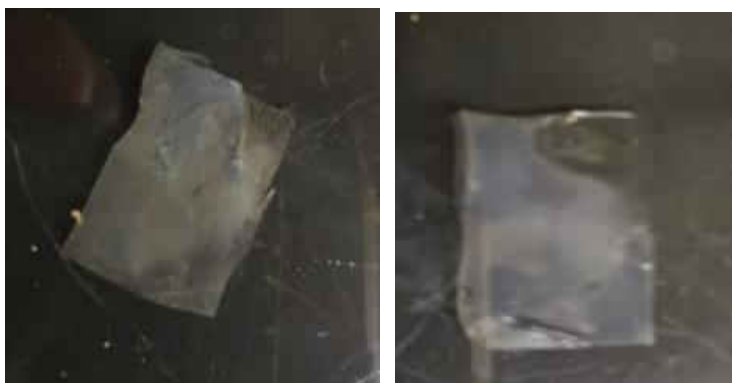
Figure 21: Untreated BNNTs on nafion (left) and acid treated BNNTs on nafion (right)
