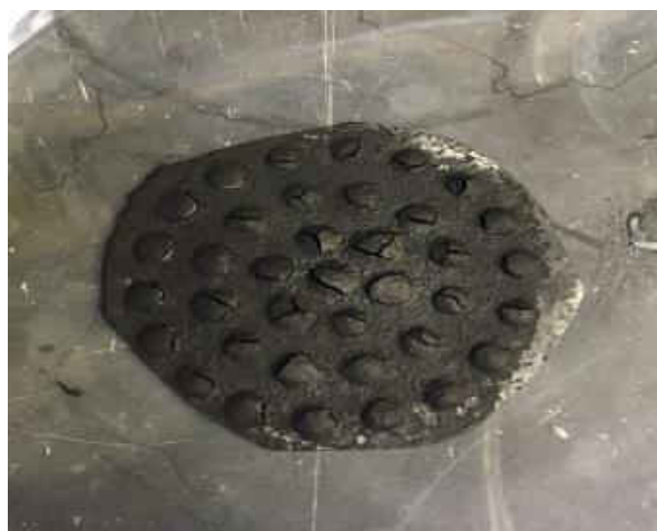
Figure 15: CNT mat after vacuum filtration
