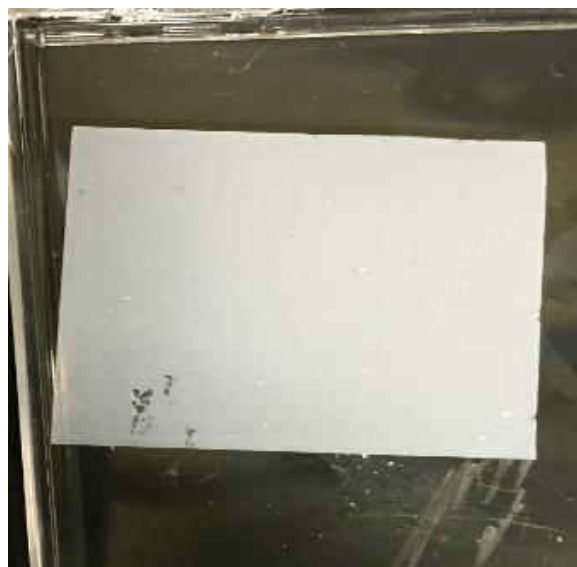
Figure 14: Nitric acid treated BNNT spray deposition
