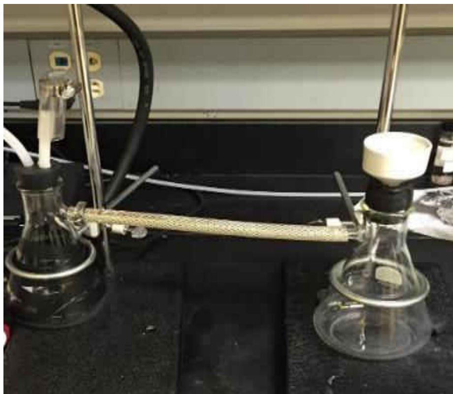
Figure 7: Vacuum filtration apparatus made for experiments
