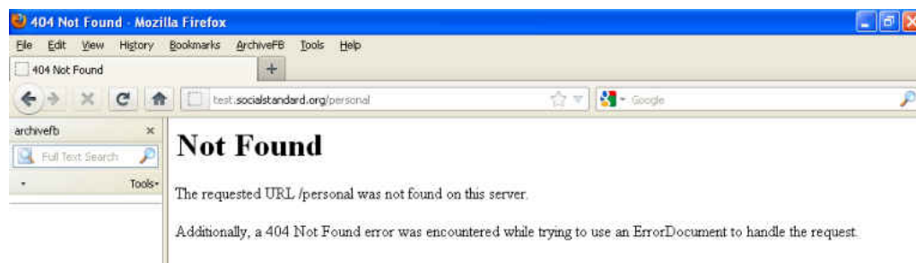
Fig. 34. The target website's URI scheme has changed. The new URI for the content that was previously at http://test.socialstandard.org/personal is now at http://test.socialstandard.org/myfeed .
