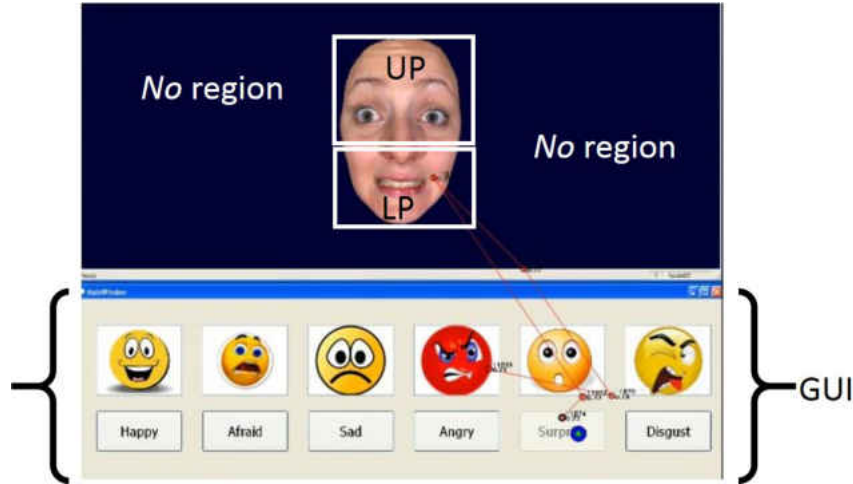
FIG. 29: Four visual areas of interest (AOI) for eye-tracking. UP and LP represent the upper and lower part of the face, respectively. GUI shows the graphical user interface region. The rest belongs to the No region .
