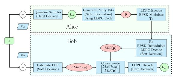
Figure 6. Proposed Key Generation Mechanism.
