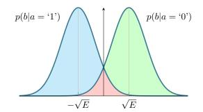
Figure 8. Conditional PDFs for a Typical Binary Receiver.
