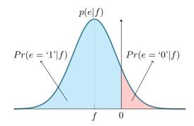
Figure 10. Channel Measurement LLR Calculation Probabilities.
