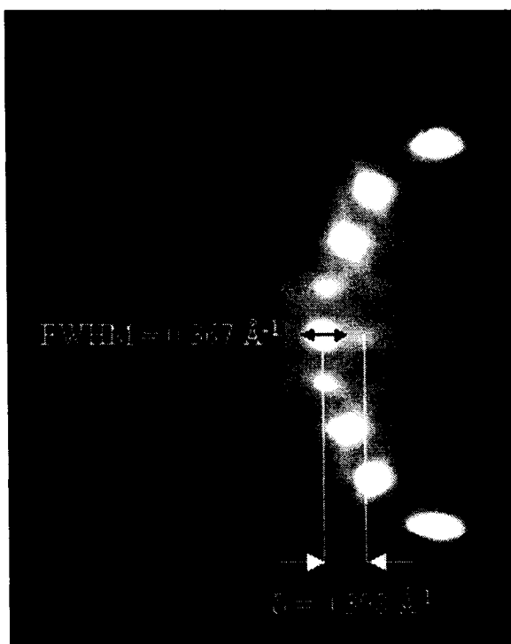
FIG. 3.13. A RHEED pattern for Si(100)-2 \times 1 used to calculate the average terrace width by calculating the splitting in the (00) peak.
