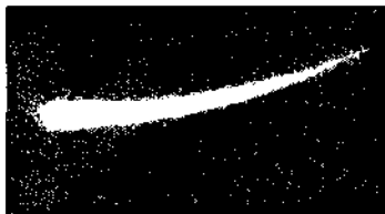
FIG. 35: An ICCD camera photograph when the plasma pencil is horizontally positioned with 3 m/s low helium flow velocity.
