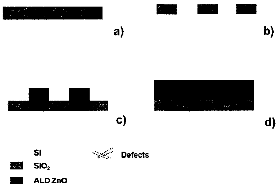
Figure 69. Proposed defect pinning in ALD ZnO on Si substrates. a) Deposition of SiO 2 layer on Si. b) Patterning of the SiO 2 Layer. c) Deposition of the ALD ZnO layer. d) defects are pinned by the SiO 2 layer.
