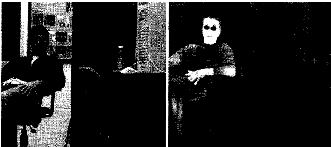
Figure 6.3. Picture on the left is captured from a visible camera and the one on the right is captured using long wave infrared camera.
