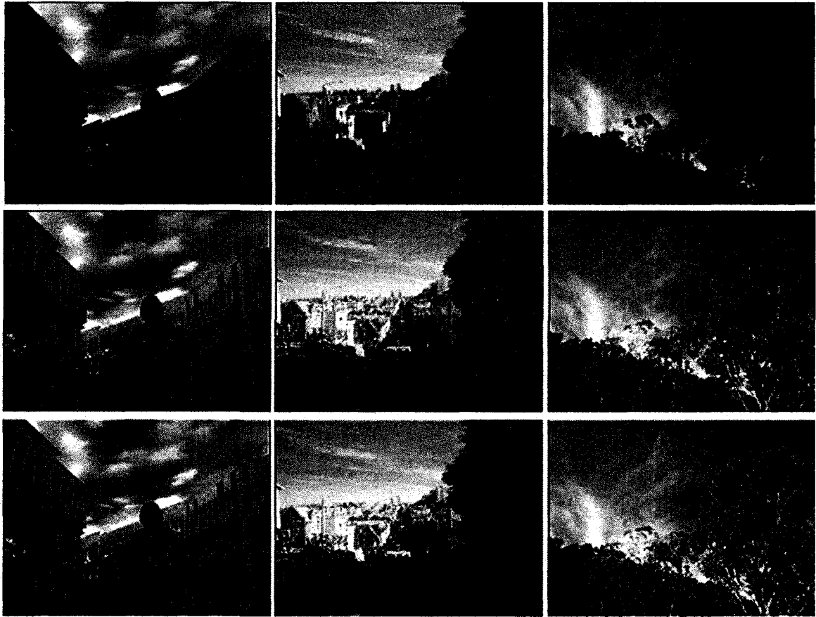
Figure 40: Images shown on 1 st row are the test color images with non-uniform darkness. Results from software and hardware simulations are illustrated on 2 nd and 3 rd rows, respectively.
