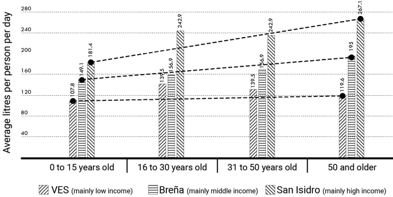
Figure 11. Relation between house age (based on survey) and water consumption (based on SEDAPAL data).
