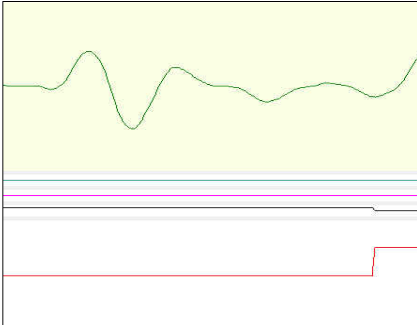
Figure 9: Screenshot of EMG onset (top pane) compared to digital trigger (bottom pane).
