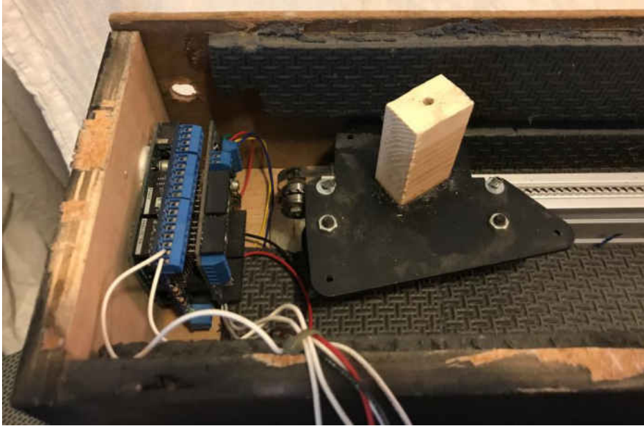
Figure 7. Close up of the Arduino computer within the IB mechanism
