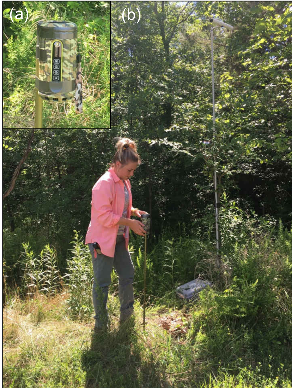
Figure 2-2. Example of acoustic detector and audio speaker deployment configuration used to assess bat response to predator cues at Wendell H. Ford Regional Training Center from June to August 2017. (a) Bliiq Infinite X Bluetooth speakers were used to broadcast audio treatments. (b) Speaker is deployed at a height of 1.5 m and is placed approximately 1.5 m from the acoustic detector microphone.
