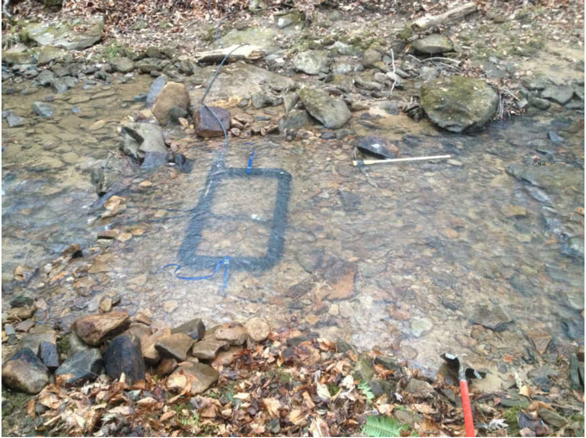
Figure 6. Kentucky Arrow Darter antenna transceiver located on Elisha Creek (antenna E7), showing placement in a naturally constricted segment of the channel.
