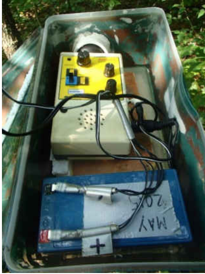
Figure 2.3. Zero-crossing acoustic detector, Anabat II system, (Titley Electronics, Colombia, MO) deployment method at Mammoth Cave National Park, Edmondson County, Kentucky, during 2010-2016. A) Anabat II detector unit housed in plastic protective case with external power source. B) Anabat II detector unit deployed 1.5 m above ground on tripod.
