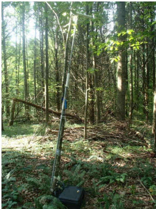
Figure 3.1. Full-spectrum acoustic detector, Songmeter SM3 (“Bat+” option, Wildlife Acoustics Inc., Maynard, MA) deployment method at Mammoth Cave National Park, Edmondson County, Kentucky, during 2015-2016. A) Songmeter SM3 unit housed in plastic protective case. B) Songmeter SM3 microphone housed in plastic protective casing and deployed 3.0 m above ground with unit at base of the tree.
