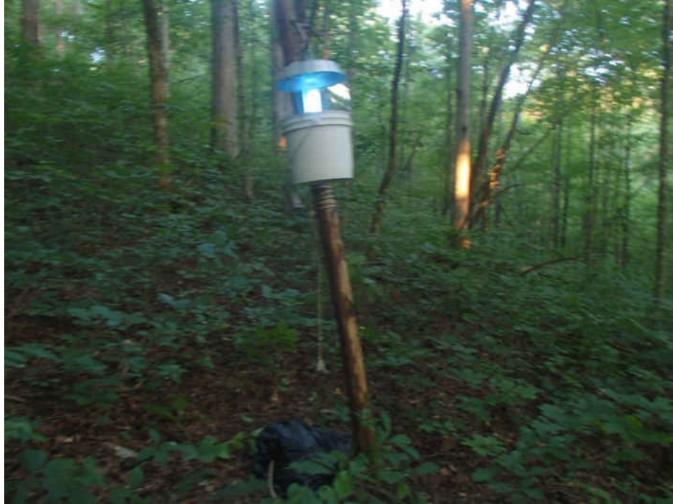
Figure 2.5. Blacklight trap deployment method for insect sampling at Mammoth Cave National Park, Edmondson County, Kentucky, during 2010-2012 and 2015-2016. Blacklight suspended 2.5 m above ground and operated from sunset to sunrise. External power source deployed in a plastic protective bag at the base of the tree.
