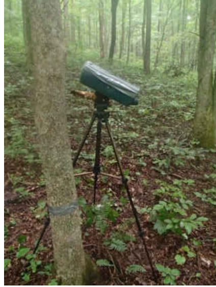
Figure 2.3. Zero-crossing acoustic detector, Anabat II system, (Titley Electronics, Colombia, MO) deployment method at Mammoth Cave National Park, Edmondson County, Kentucky, during 2010-2016. A) Anabat II detector unit housed in plastic protective case with external power source. B) Anabat II detector unit deployed 1.5 m above ground on tripod.
