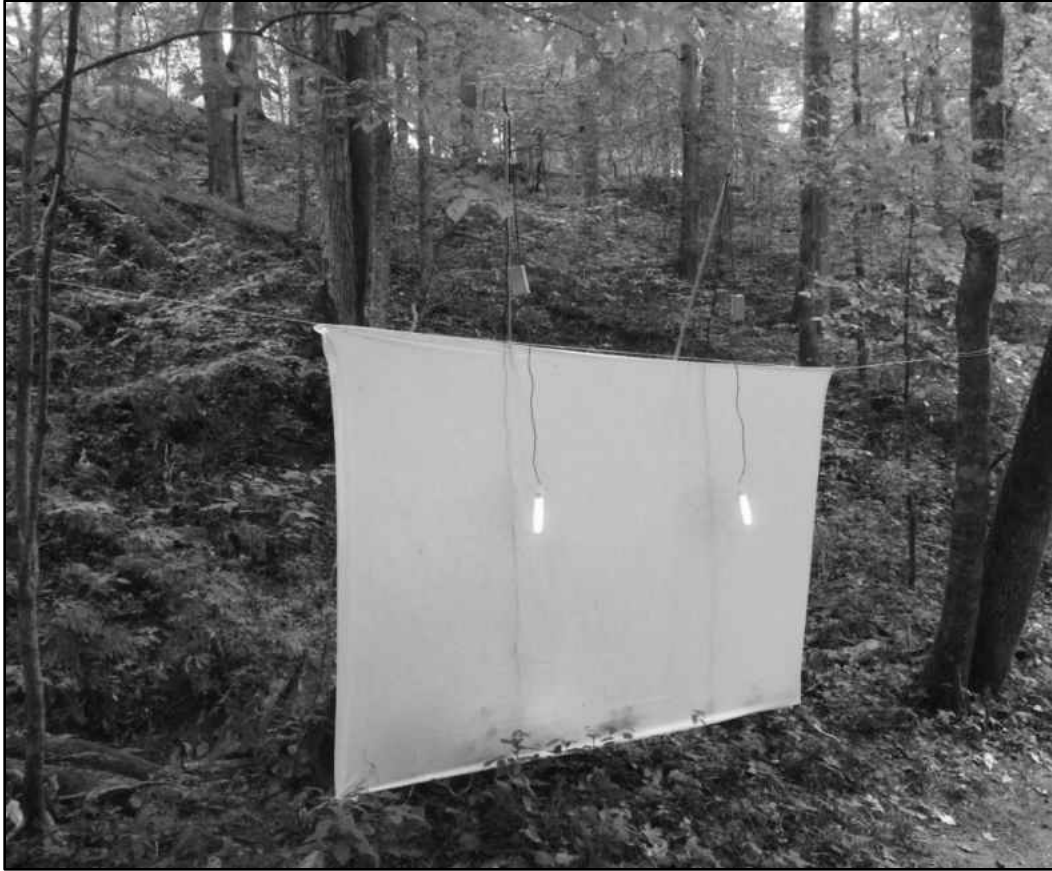
Figure 1.1. Cotton sheet deployed at Mammoth Cave National Park to sample Lepidoptera, illuminated by 10-W black lights with electrical harnesses.
