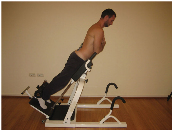
Figure 2. The tilting device used for testing with subject placed in starting position.
