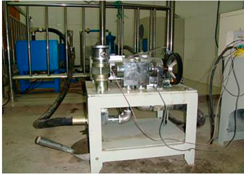
Figure 3. Grouting test system.
