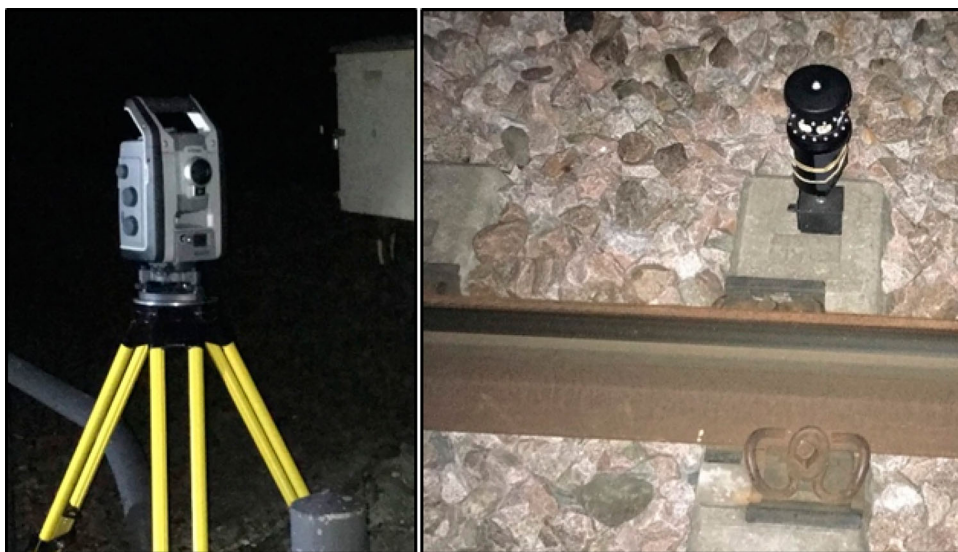
Figure 1. Total station and active prism.
