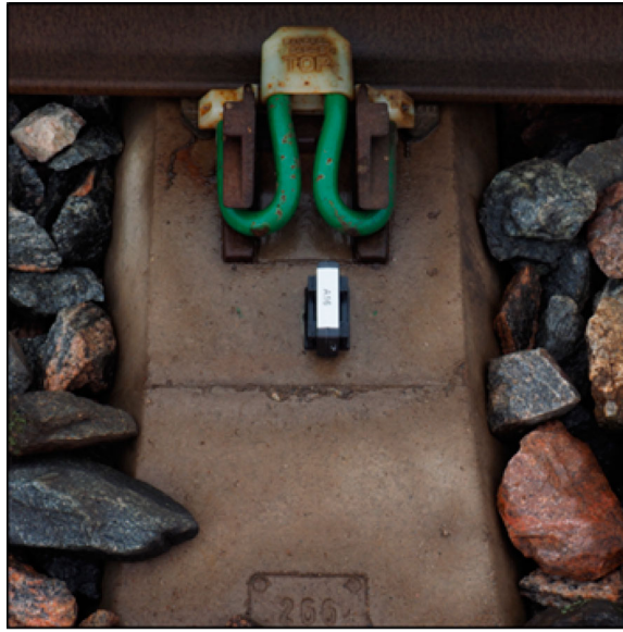
Figure 2. Stand-alone MEMS accelerometer used for deflection and stiffness survey deployed on a sleeper end.
