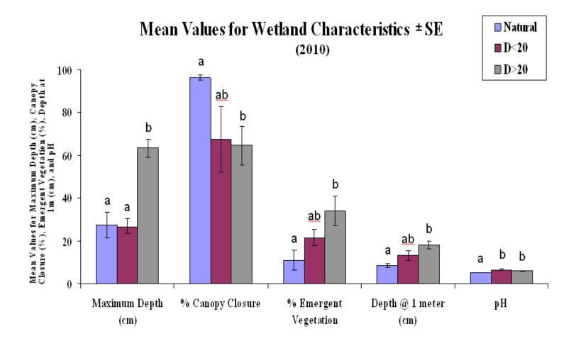
Figure B-8. Mean values for wetland characteristics  $\pm$  standard error by wetland type [(natural, shallow constructed (D < 20), deep constructed (D > 20)] for 2010. Different letters indicate statistical significance between groups and shared letters indicate lack of statistical significance between groups.
