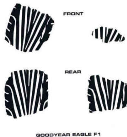
Figure 2.12: Vehicle at Turn Tire Patches
