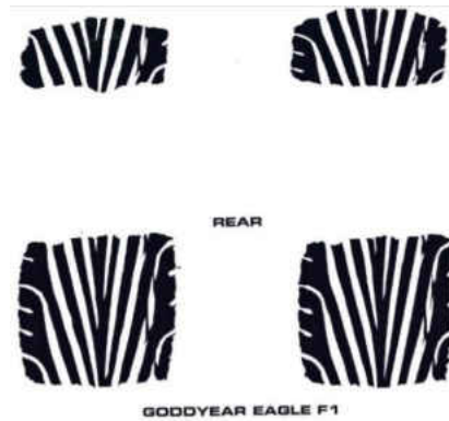
Figure 2.10: Vehicle at Acceleration Tire Patches
