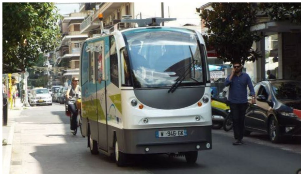
Figure 1. Automated shuttle by Robosoft on a public road in a mixed traffic situation in Trikala, Greece.
