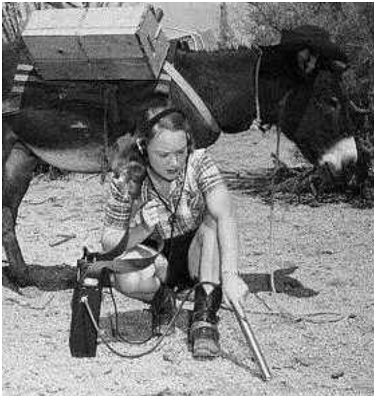
Figure 12: National Geographic photo of a woman operating a Geiger counter, 1953. Source: Robert Nininger, "When rock blooms yellow and Geiger counter rattle – uranium!" National Geographic Society , June, 1953.
