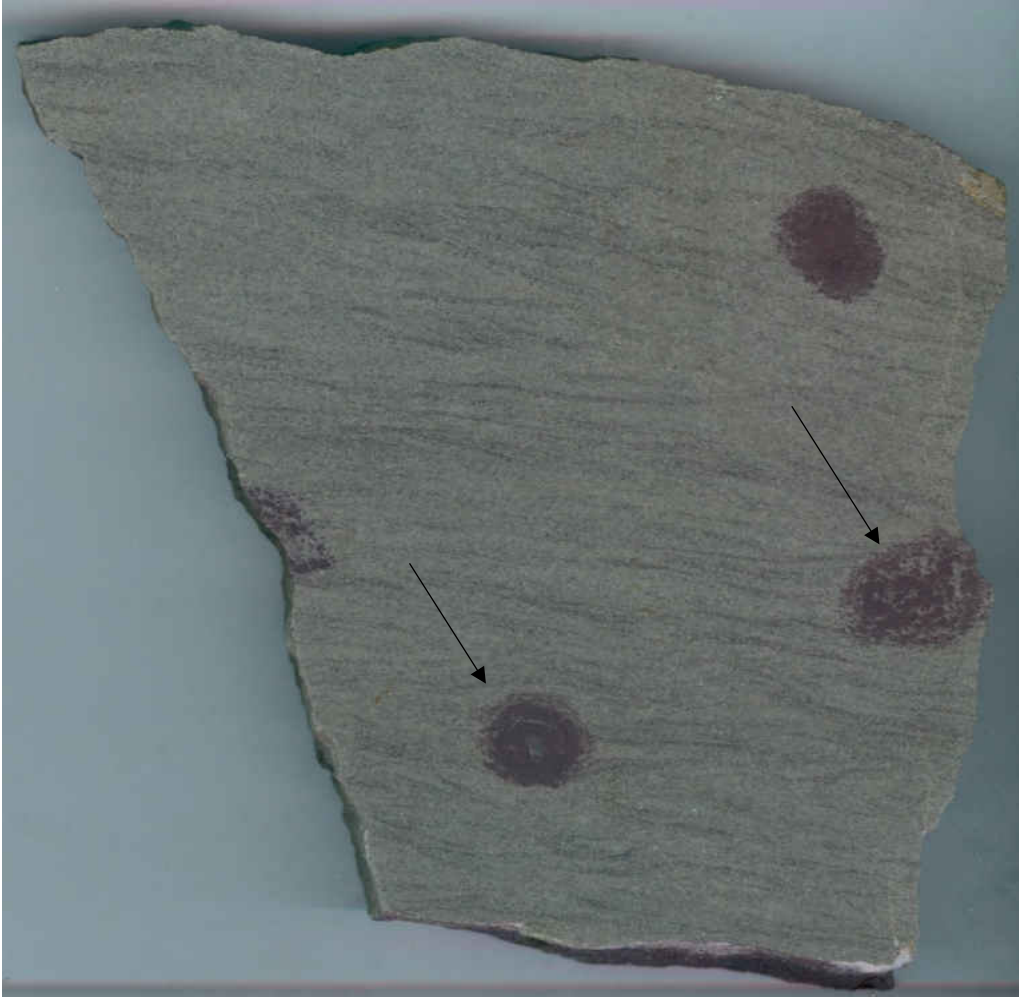
CI-D: Light-gray sandstone collected from 29.19 m within Upward-coarsening Sequence 2 (lithologic unit 16). Exhibits internal lamination with thin mud drapes and discrete horizontal burrows ranging in size from 0.6 cm to 1.3 cm in diameter.
