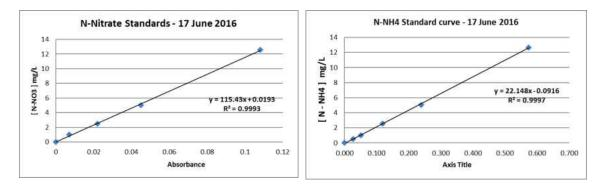
Figure 4. Typical calibration curves for nitrate and ammonium showing best-fit parameters and r2 values.
