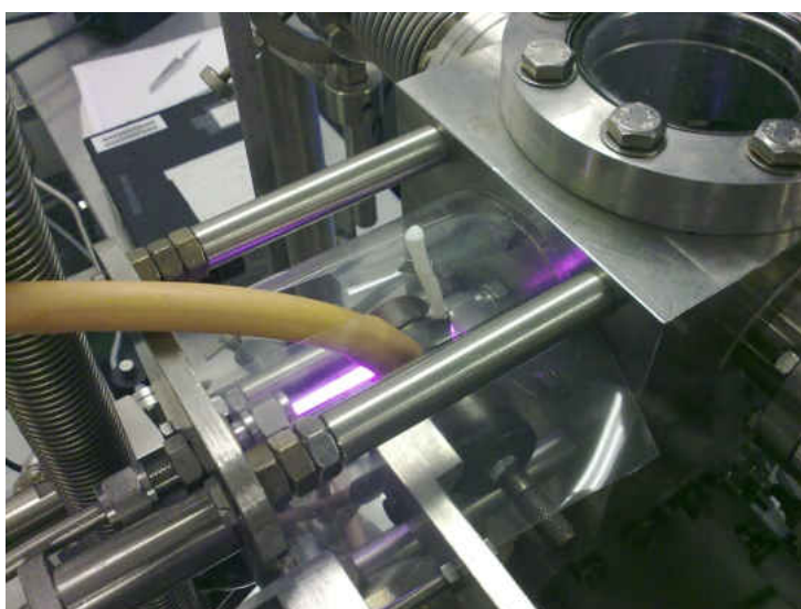
Figure 3.13 Microwave plasma source in operation. The resonance cavity is at the centre of the image with the Pyrex capillary (with glowing plasma) set through the middle. The orange tubing is the cooling air supply. The load lock loading window can be seen at the top-right.
