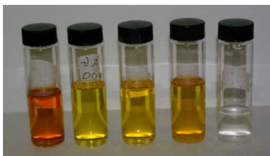
Figure 3.1: Samples were produced by dip-coating the substrate into the relevant sol, and this photo shows some of these sols. Left to right: zirconia containing yttria nanoparticles (not used), 2.04 mol% yttria (recipe A), 4.17 mol% (recipe B), 19.1 mol% (recipe D), and yttrium nitrate dissolved in water. Photo: Matt Gunn.
