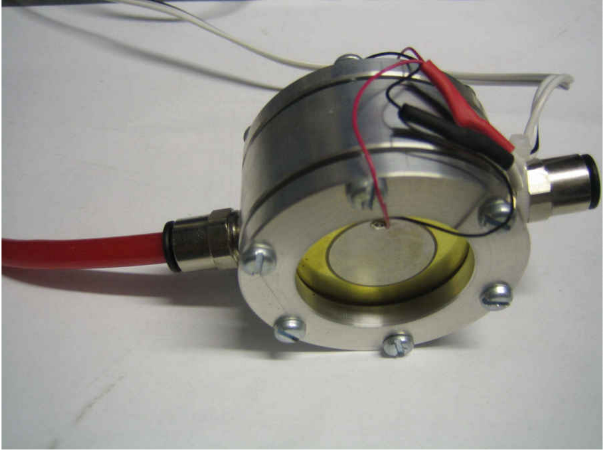
Figure 4.6: Built double-piezo used to generate acoustic waves of variable frequencies controlled via a frequency generator.
