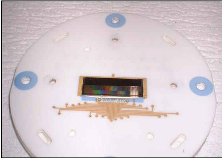
Figure 2.7: Detector array on ceramic substrate
