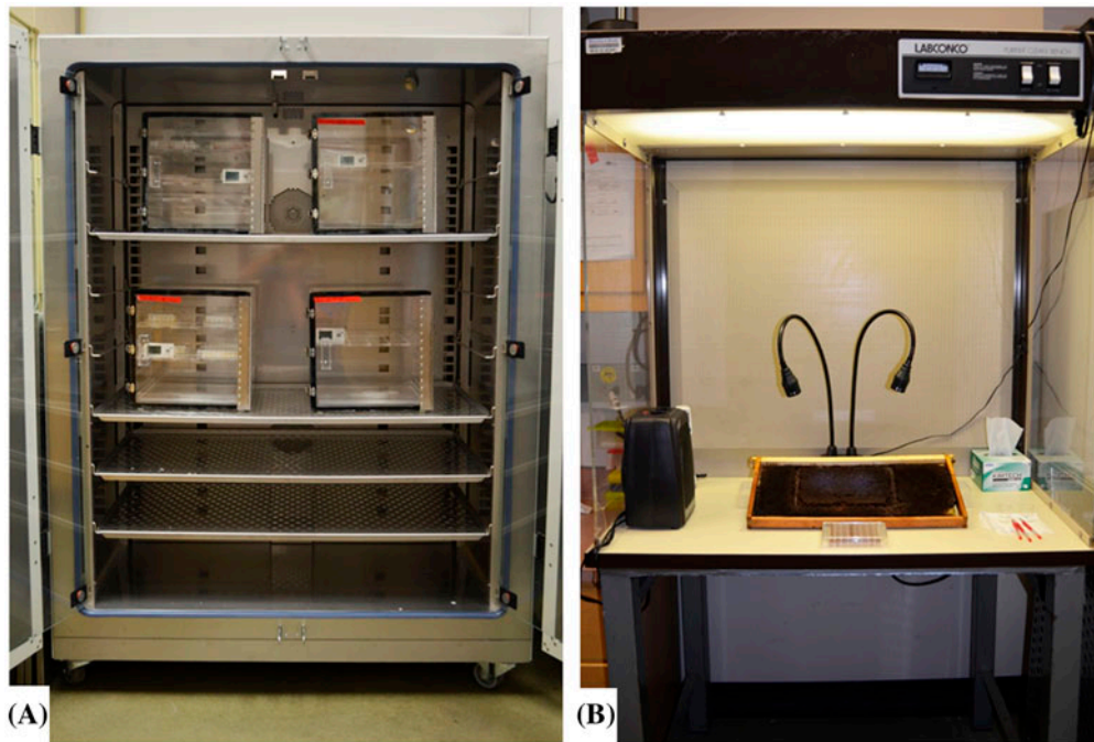
Figure 3. Incubator containing desiccators used to house larval and pupal sterile tissue culture plates (A), and positive flow hood used for in vitro larval grafting, feeding, and monitoring for mortality (B).
