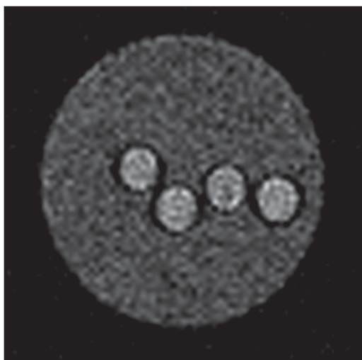
Figure 5. T_1 -weighted spin-echo MRI image (measured at 1T) of an agar phantom containing TS/A cells grown in: normoxia, hypoxia, 225 mOsm, medium, 300 mOsm medium (from the left to the right, respectively).
