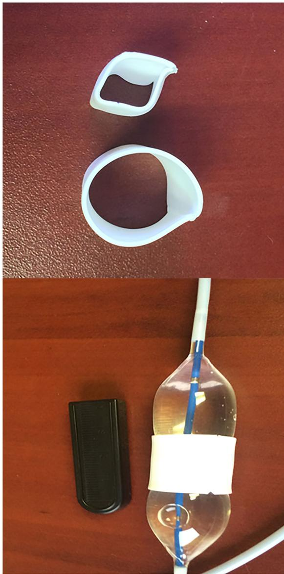
**Figure 1.** In vitro benchtop balloon dilation of the anisotropic (test) conduit. A 10 mm test conduit is dilated with a 20 mm catheter based balloon to its final diameter of 21.5 mm. Wall tension was not calculated during this test. The black thumb drive is in the image for perspective, measuring 4.5 cm x 1.5 cm.
