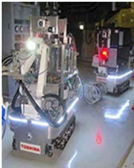
Figure 51 - Dry Ice Blast Decontamination Robot (TEPCO 2016)
