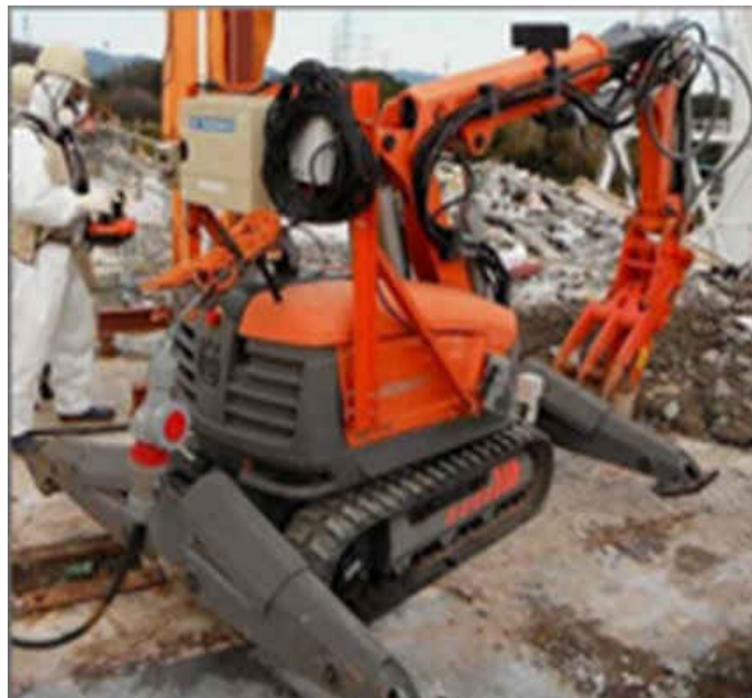
Figure 52 - Floor Decontamination Robot (TEPCO 2016)
