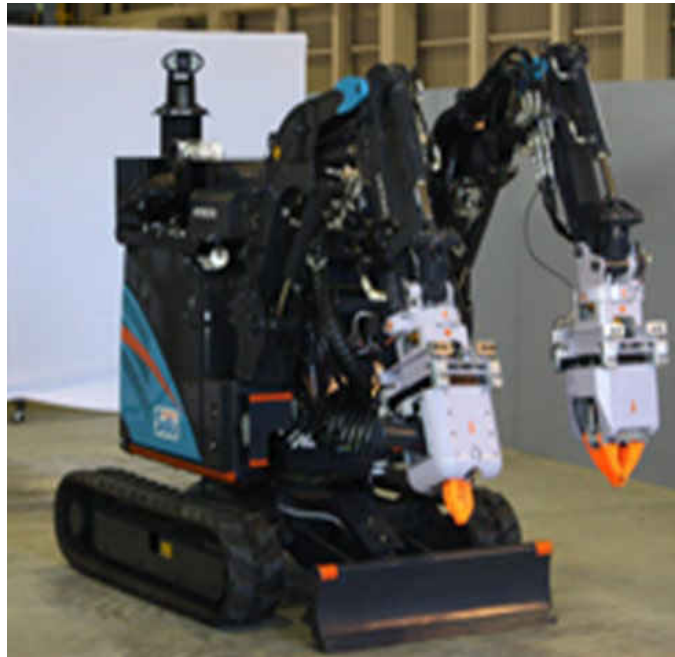
Figure 55 - Debris Removal Robot (ASTACO-SoRa) (TEPCO 2016)
