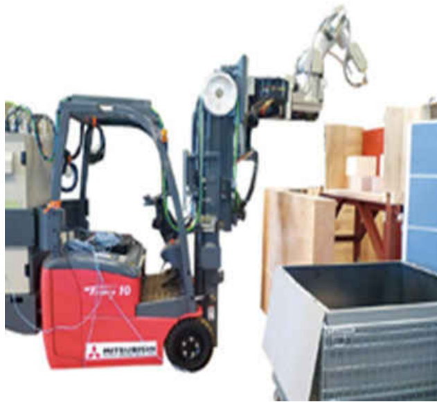
Figure 48 - Used to Remove Shielding Blocks (TEPCO 2016)
