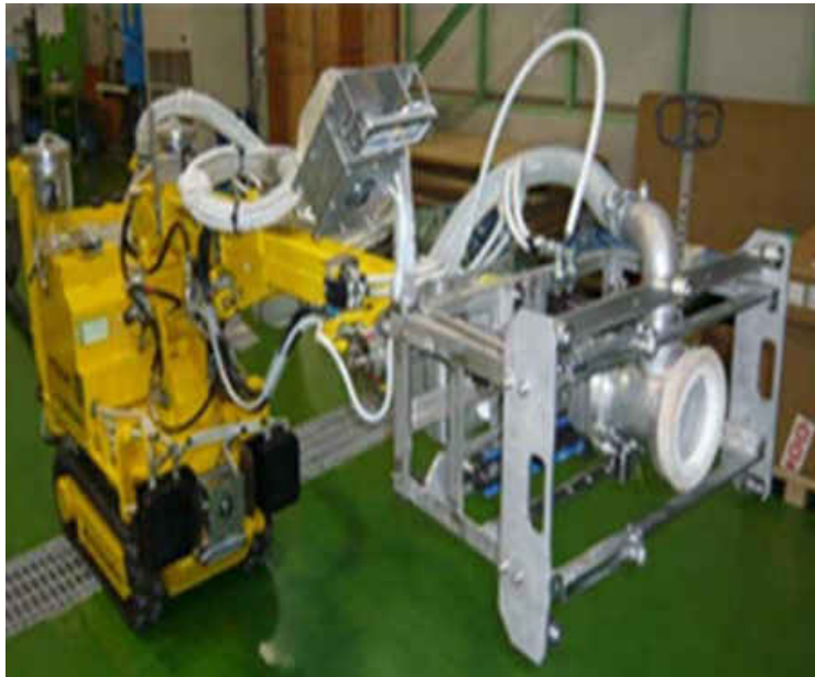
Figure 49 - High Pressure Decontamination Robot (TEPCO 2016)
