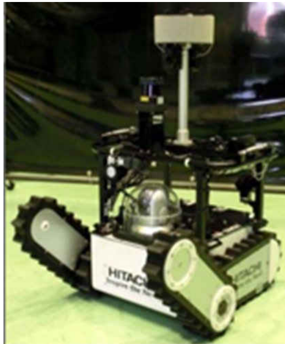
Figure 53 - 3D Laser Scanning Robot (TEPCO 2016)
