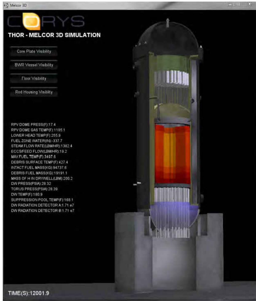
Figure 20 – Corys Thunder MELCOR Simulation (Sanders and Panfil 2013)
