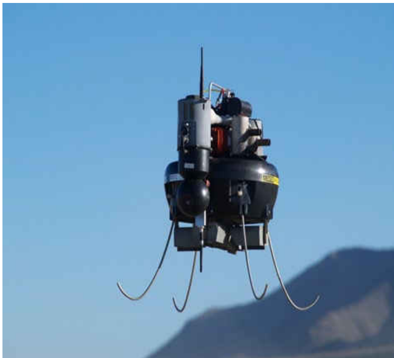
Figure 67 - Honeywell T-Hawk MAV (Aerospace 2009)
