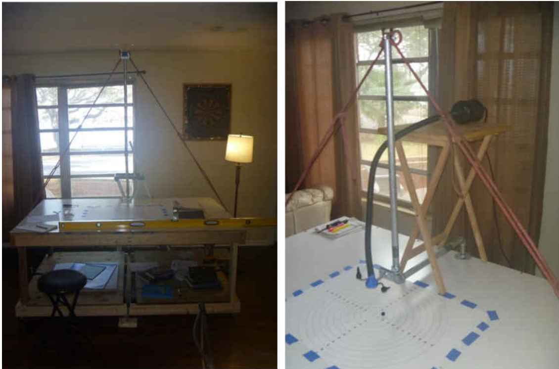
Figure 18. Experimental laboratory setup. Left picture shows the configuration for experiment 1 (55 to 22 inch heights). Right picture shows the configuration used for 38 inch heights and lower.
