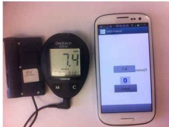
Figure 5 Data transfer from glucose meter to SAED application(Alotaibi, Istepanian, Sungoor, & Philip, 2014a)
