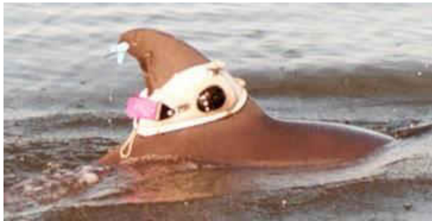
Figure 3. Instrumented Trac-Pac on dorsal fin of FB984 in the Indian River Lagoon (2004).
