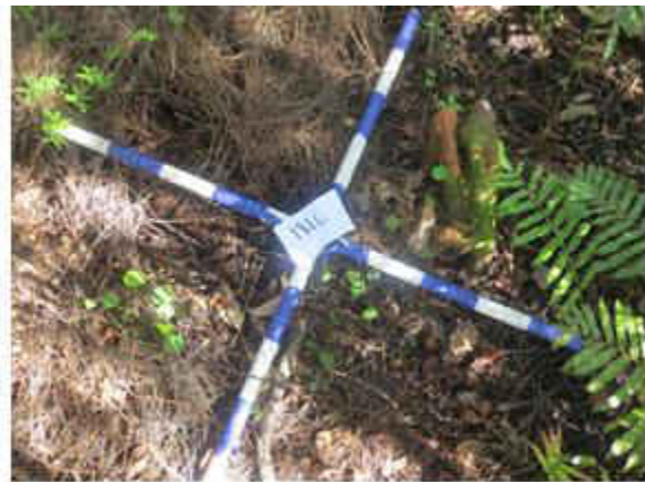
Figure 28: Example of PVC quadrat used in the field for estimating species percent cover.
