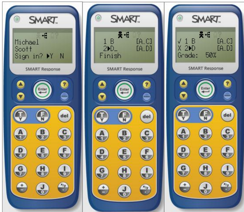
Figure 10: The progression of a student signing in, inputting their answers, and the feedback sent through a SMART Clicker.
